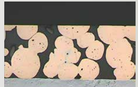
Fig. 8: Condition of sliding surface during service life
