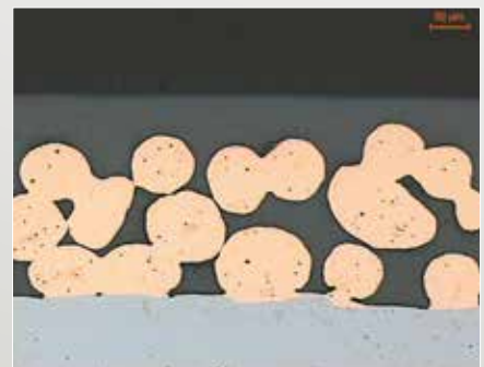
Fig. 4: Condition of sliding surface in the initial state
