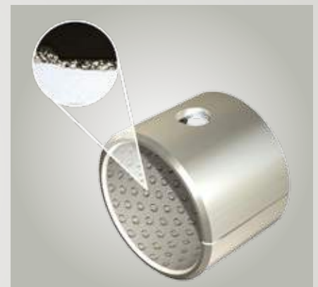
Fig. 21: P200 plain bearing with oil distributing pocket and oil hole
