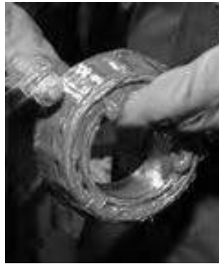
Fig. 23. Grease can easily be packed by hand.
